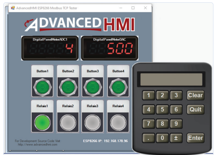
Figure 2: The AdvancedHMI software generates human-machine interface applications.
