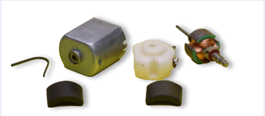
Figure 1: The component parts of a fractional horsepower DC motor. The commutator is clear to see on the rotor shaft by the armature coils. (Source: Shutterstock/Pixel Enforcer)
