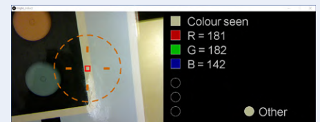
Figure 11: Misclassification of other colors as 'green' resolved using 'other' output node.
