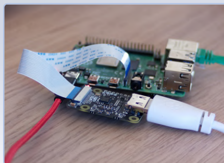
Figure 18: Finished setup with HDMI-to-CSI bridge.
