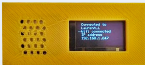
Figure 5: A wireless serial debug unit complete with 3D-printed case.
