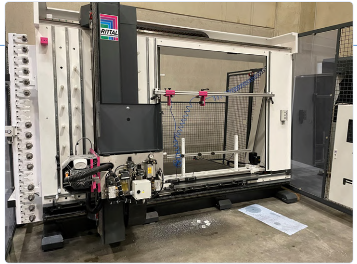
Figure 1: Industrial cutter from FEGA & Schmitt with monitoring. (Source: Würth Elektronik eiSos)
