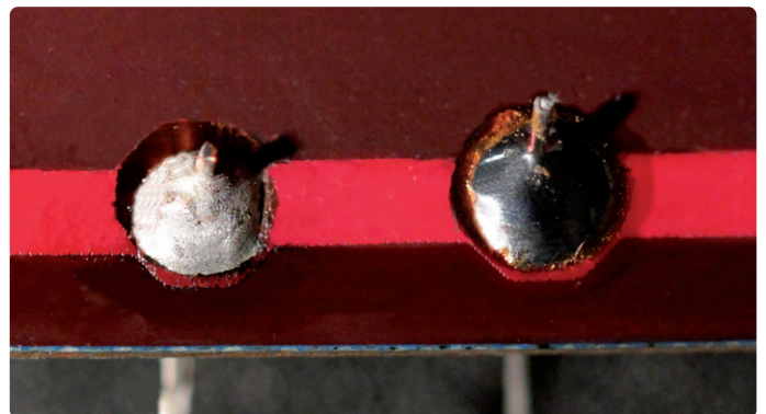
Figure 3: Different appearances: a lead-free solder joint (left) and a conventional lead solder joint (right).
