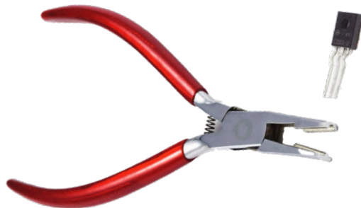
Figure 17: To avoid stress from thermal expansion, the leads of the driver transistors are bent slightly. This can be done very easily with the special pliers shown here, but it can also be done with round-nose pliers.
