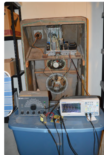
Figure 10: The low-Q amplifier used to measure the frequency of a loop antenna on an antique console radio.
