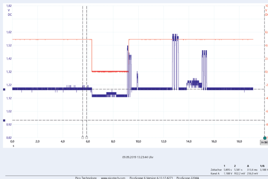
Figure 1: The 433 MHz band is very busy. Signals from different transmitter modules are shown here. The pulse sequence in the middle is the one we want.
