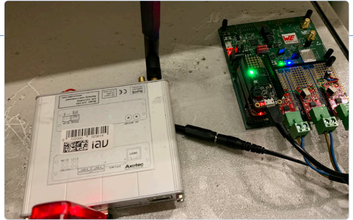
Figure 5: Current measurement using a Hall-effect sensor. (Source: Würth Elektronik eiSos)
