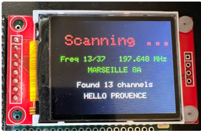
Figure 6: Here we see that the multiplex MARSEILLE 8A is found and that it contains 13 stations.
