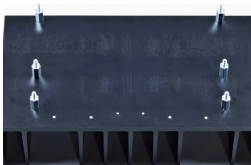
Figure 12: The marked locations of the drilled holes for mounting the power transistors.
