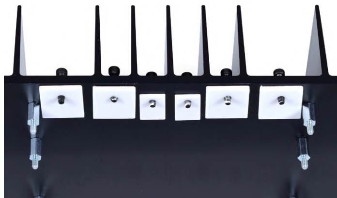
Figure 21: The ceramic pads are coated on one side with a thin layer of thermal paste and fitted over the partially-inserted screws. The heat sink must be positioned upright for this.
