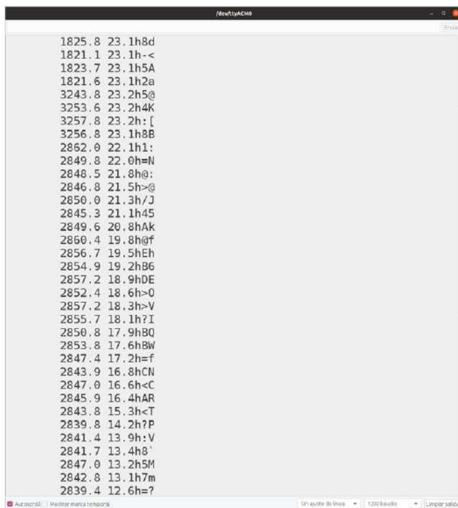
▲ Figure 7: Arduino's Serial Monitor displaying DDI messages from TEROS 11.
