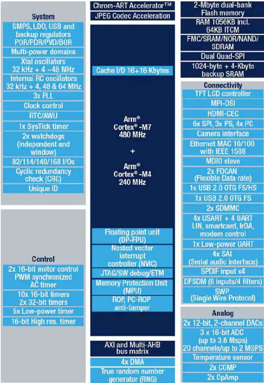
Figure 8: Overview STM32H747XI. (Source: STMicro, https://bit.ly/3xoRTDF )
