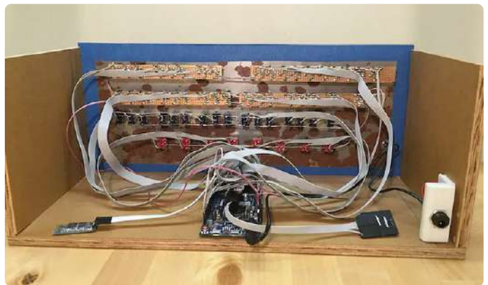
Figure 6: Inside view of the Arduino Altair clone.
