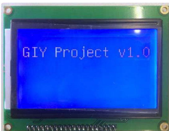
Figure 9: The LCD used has a resolution of 128x64 pixels and is connected to the board using only 3 pins.
