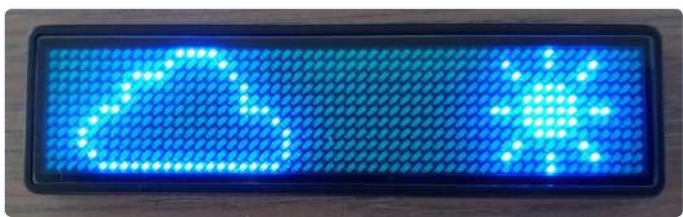
Figure 6: By sending the appropriate BLE commands, you can show off your very own 11 × 55 pixel images on the LED badge.
