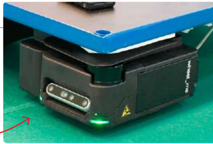
A wheel.me autonomous wheel does heavy lifting intelligently.
