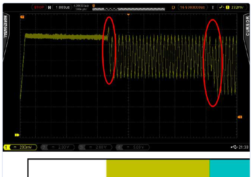
Figure 17: Phase changes during color change are marked.
