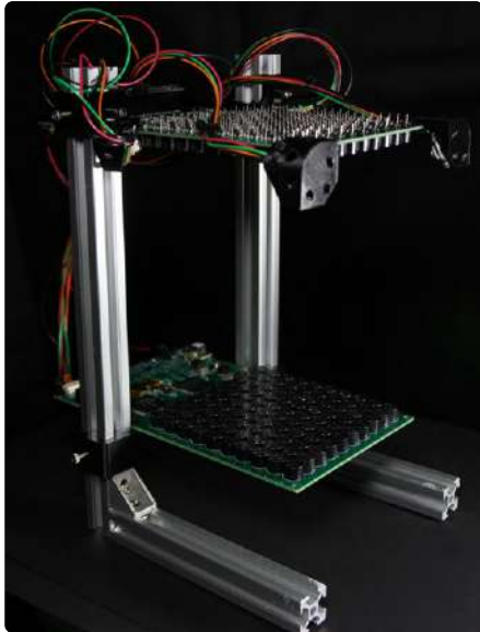
Figure 1: Two arrays, each consisting of 100 ultrasonic transducers, are used to make a small foam ball float in the air.
