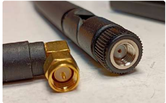
Figure 2: Antennas with SMA connectors. Left is right and right is wrong for Opera Cake and HackRF One.
