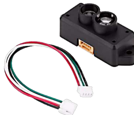
Figure 1: The low-cost TFMMini-S LiDAR features a range of 12 m with a resolution of 1 cm.
