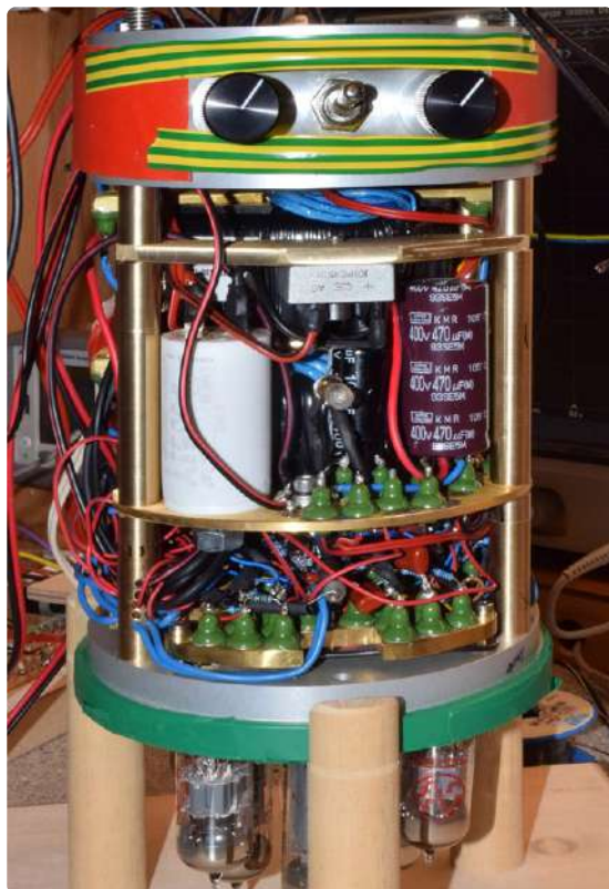
Figure 17: Provisional assembly of the complete amplifier, without the protective tubular enclosure.
