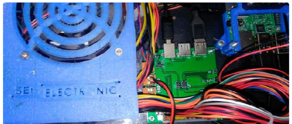
Figure 4: ATX power supply connected to the PCB.
