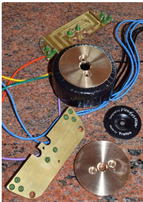
Figure 15: A round transformer for a round amplifier. Here, as well, additional mechanical parts are required for fixing.
