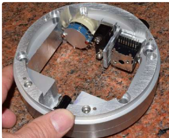
Figure 16: The user interface components (selector switch, power switch and loudness potentiometer) are mounted on their own aluminum ring.
