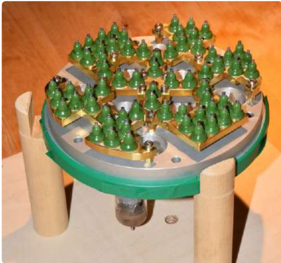
Figure 12: Solder posts with nearly vintage green glass insulators.
