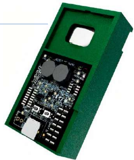
Figuur 3: SLN-LOCAL2-IOT offline spraakaansturingsoptelling van NXP. (Bron: NXP [10])
