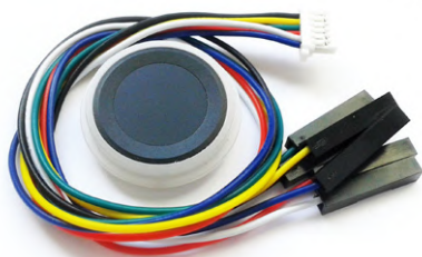
PIN1: V_Touch, 3.3V PIN2: Touch Out PIN3: VCC, 3.3V PIN4: TX PIN5: RX PIN6: GND
