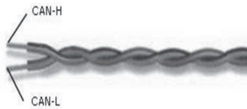
Figure 2.6 CAN is a two-wire bus
