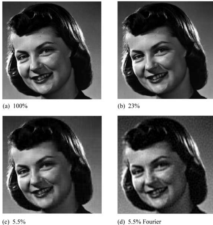
Figure 13.10.5. (a) IEEE test image, 256 \times 256 pixels with 8-bit grayscale. (b) The image is transformed into the wavelet basis; 77% of its wavelet components are set to zero (those of smallest magnitude); it is then reconstructed from the remaining 23%. (c) Same as (b), but 94.5% of the wavelet components are deleted. (d) Same as (c), but the Fourier transform is used instead of the wavelet transform. Wavelet coefficients are better than the Fourier coefficients at preserving relevant details.
