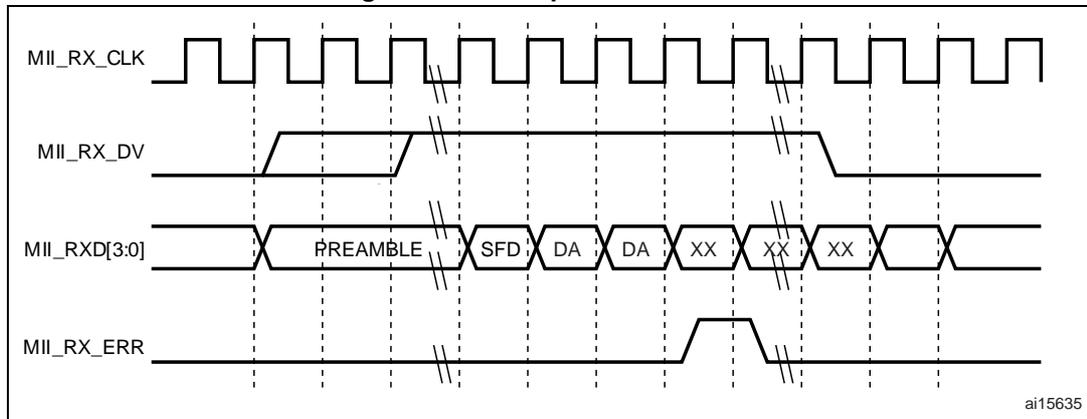
Figure 369. Reception with false carrier indication
