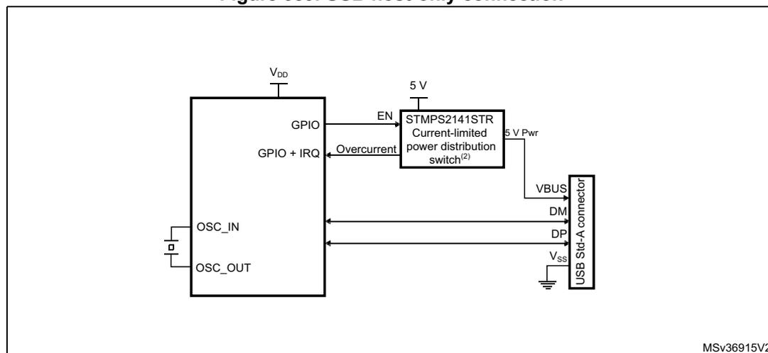
1. STMP52141STR needed only if the application has to support a  $V_{BUS}$  powered device. A basic power switch can be used if 5 V are available on the application board.
