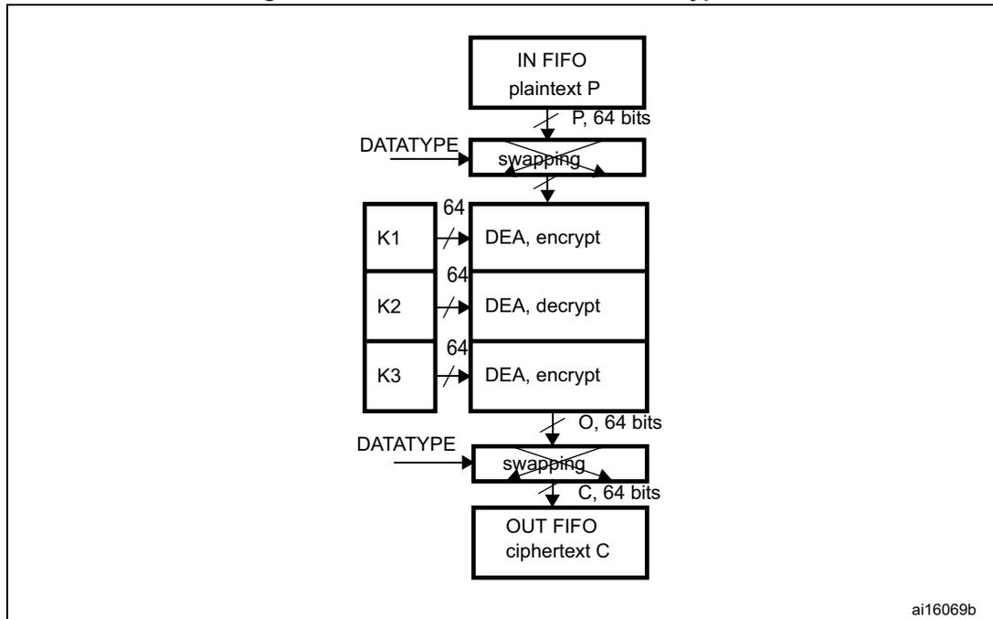
1. K: key; C: cipher text; I: input block; O: output block; P: plain text.
