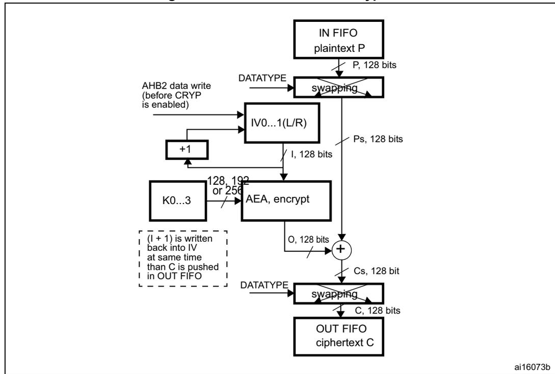
1. K: key; C: cipher text; I: input Block; o: output block; Ps: plain text before swapping (when decoding) or after swapping (when encoding); Cs: cipher text after swapping (when decoding) or before swapping (when encoding); P: plain text; IV: Initialization vectors.
