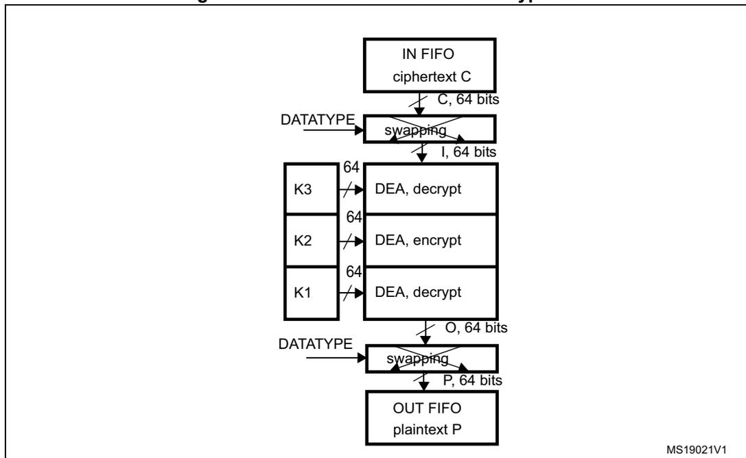
1. K: key; C: cipher text; I: input block; O: output block; P: plain text.
