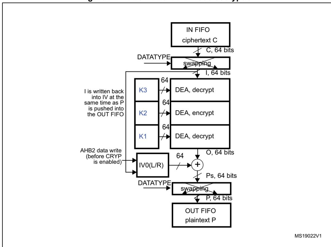
1. K: key; C: cipher text; I: input block; O: output block; Ps: plain text before swapping (when decoding) or after swapping (when encoding); P: plain text; IV: initialization vectors.
