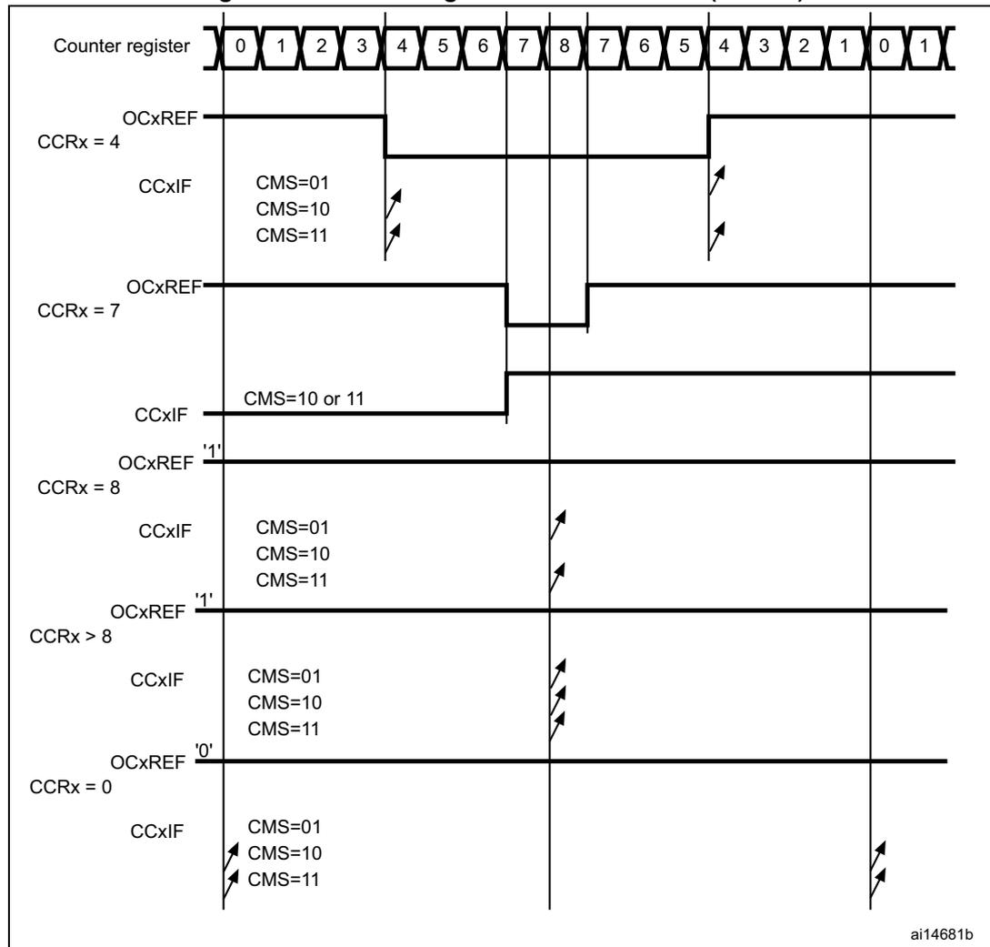
Hints on using center-aligned mode:
