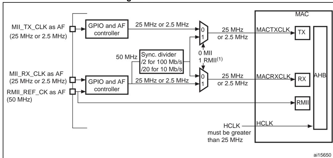
1. The MII/RMII selection is controlled through bit 23, MII\_RMII\_SEL, in the SYSCFG\_PMC register. To save a pin, the two input clock signals, RMII\_REF\_CLK and MII\_RX\_CLK, are multiplexed on the same GPIO pin.
