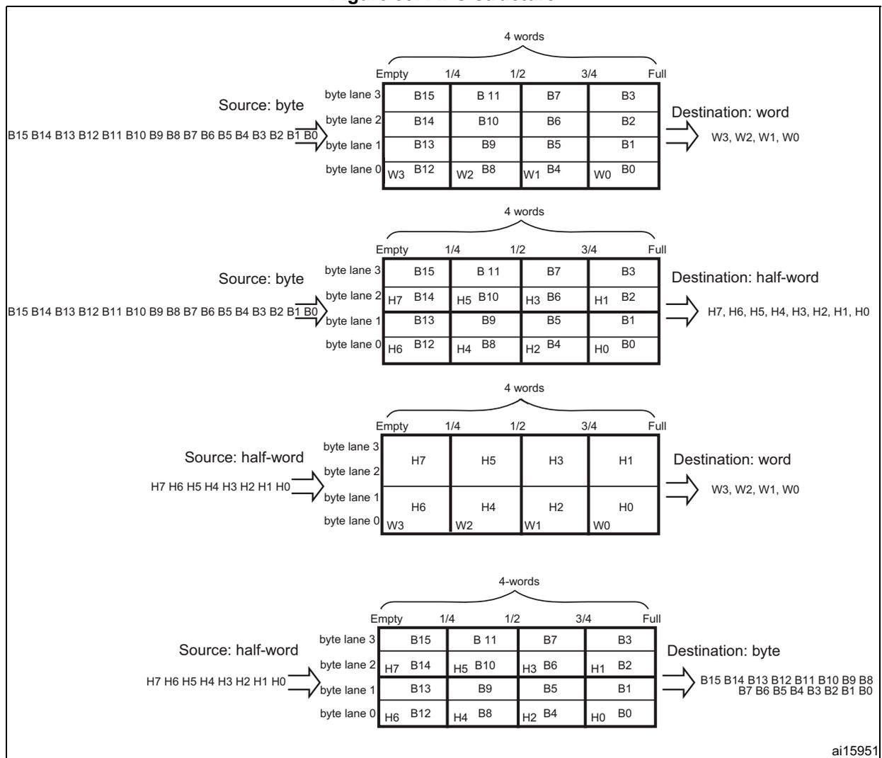
**FIFO threshold and burst configuration**
