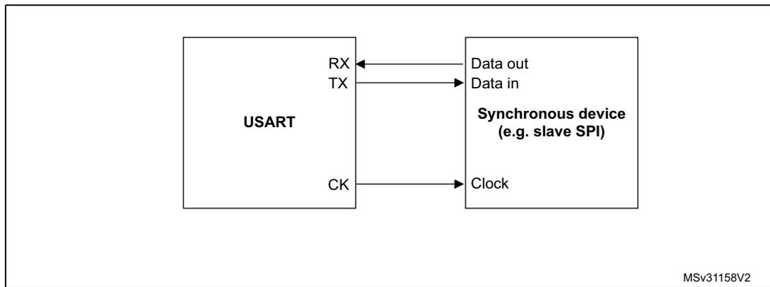
Figure 308. USART data clock timing diagram (M=0)
