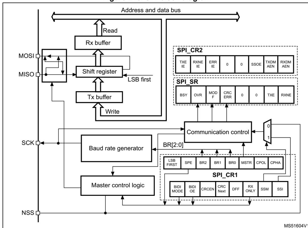
Usually, the SPI is connected to external devices through four pins:
