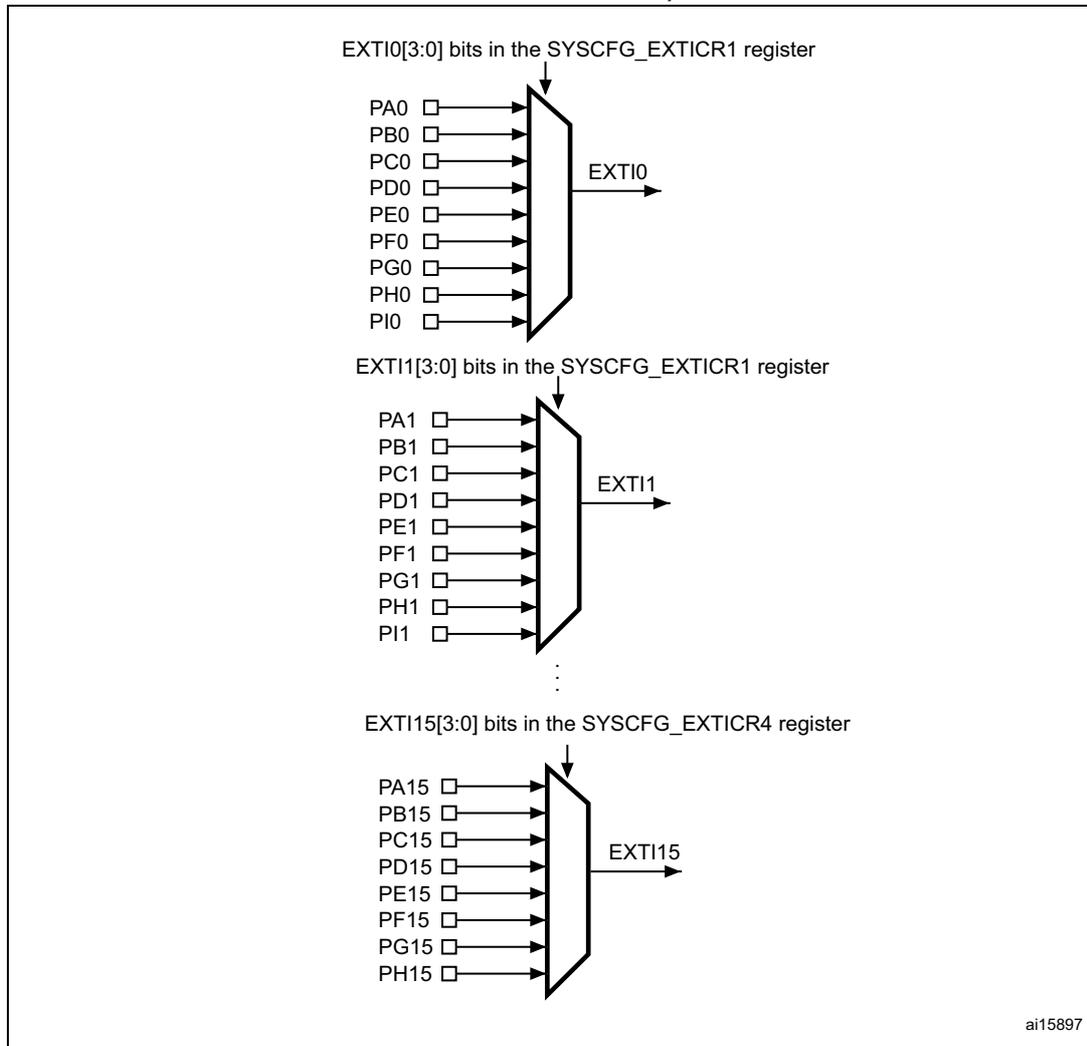
**Figure 43. External interrupt/event GPIO mapping (STM32F42xxx and STM32F43xxx)**
