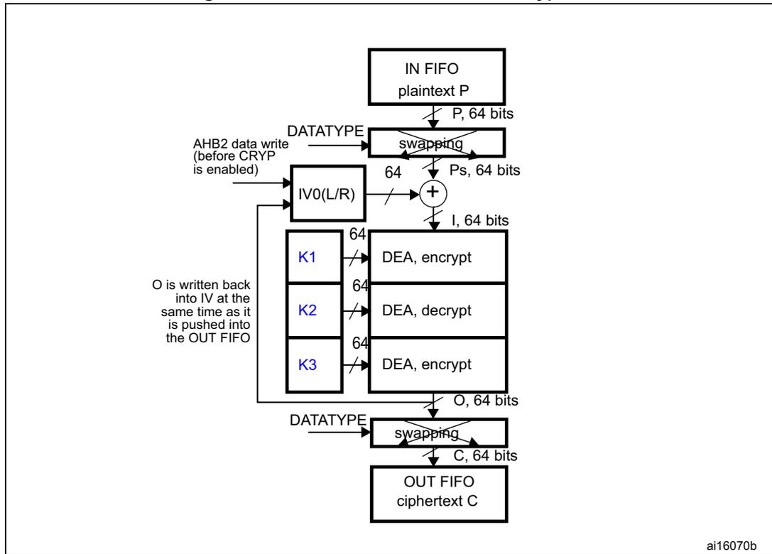
1. K: key; C: cipher text; I: input block; O: output block; Ps: plain text before swapping (when decoding) or after swapping (when encoding); P: plain text; IV: initialization vectors.
