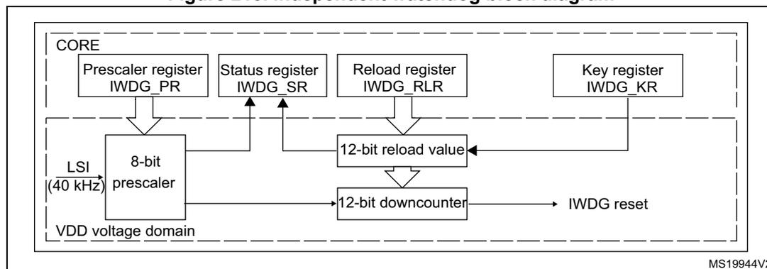
Note: The watchdog function is implemented in the V<sub>DD</sub> voltage domain, still functional in Stop and Standby modes.
