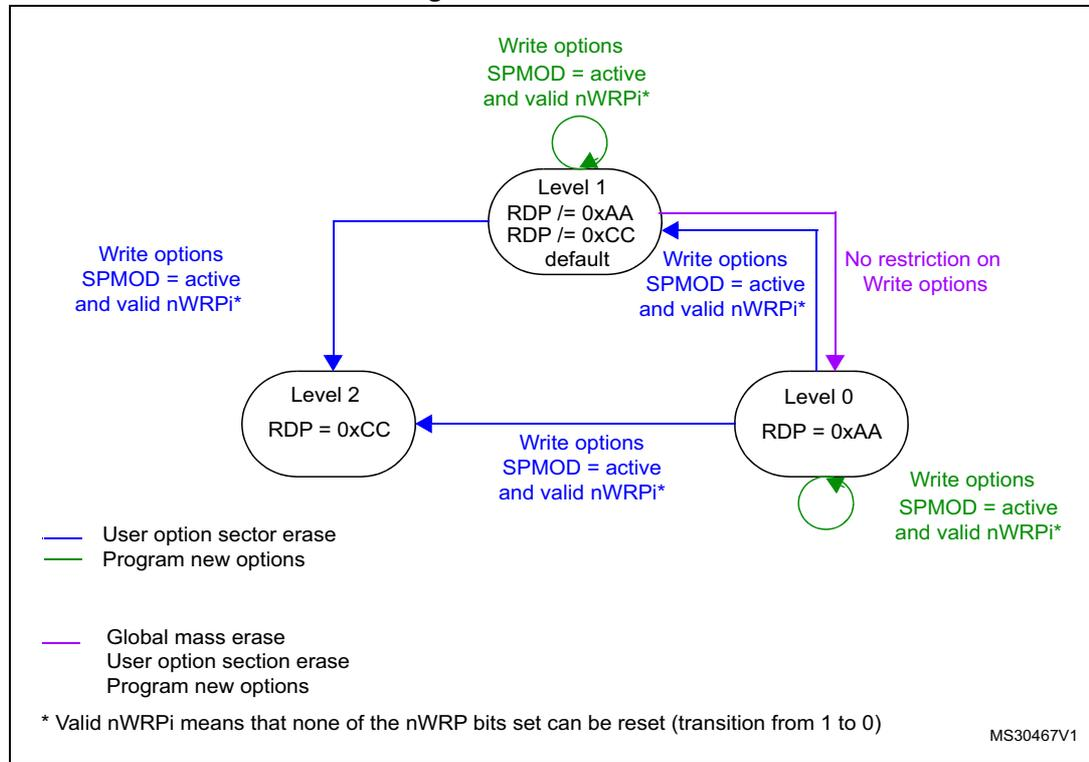
The deactivation of the SPRMOD and/or the unprotection of PCROPed user sectors can only occur when, at the same time, the RDP level changes from 1 to 0. If this condition is not respected, the user option byte modification is cancelled and the write error WRPERR flag is set. The modification of the users option bytes (BOR\_LEV, RST\_STDBY, ..) is allowed since none of the active nWRP<sup>i</sup> bits is reset and SPRMOD is kept active.
