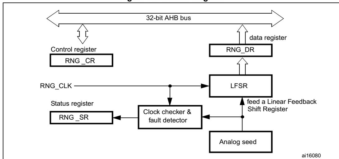
1. For more details about RNG Clock (RNG\_CLK) source, please refer to [Section 6: Reset and clock control for STM32F42xxx and STM32F43xxx \(RCC\)](#) and [Section 7: Reset and clock control for STM32F405xx/07xx and STM32F415xx/17xx\(RCC\)](#).
