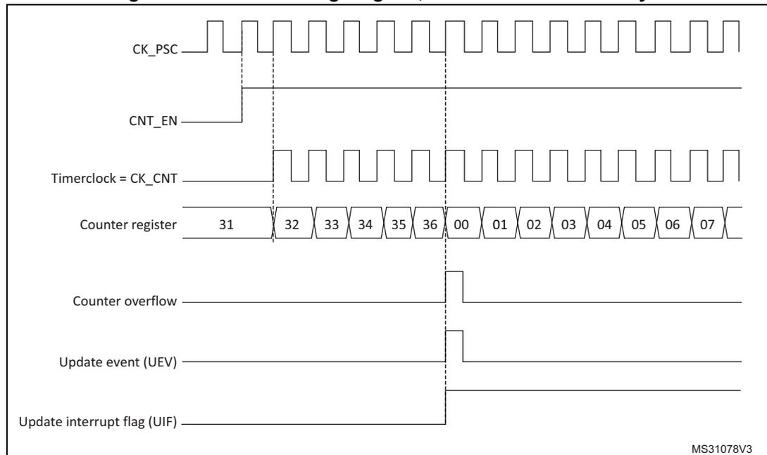
**Figure 90. Counter timing diagram, internal clock divided by 2**
