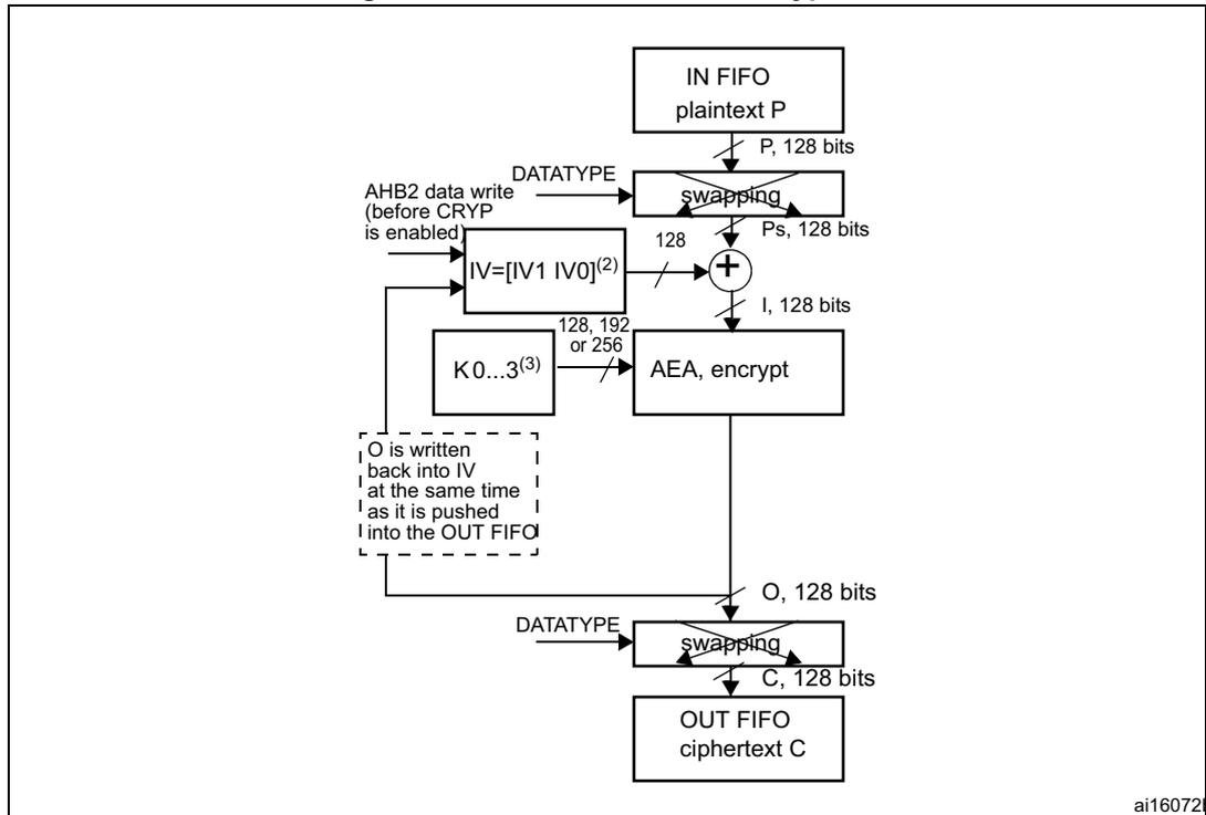
1. K: key; C: cipher text; I: input block; O: output block; Ps: plain text before swapping (when decoding) or after swapping (when encoding); P: plain text; IV: Initialization vectors.
