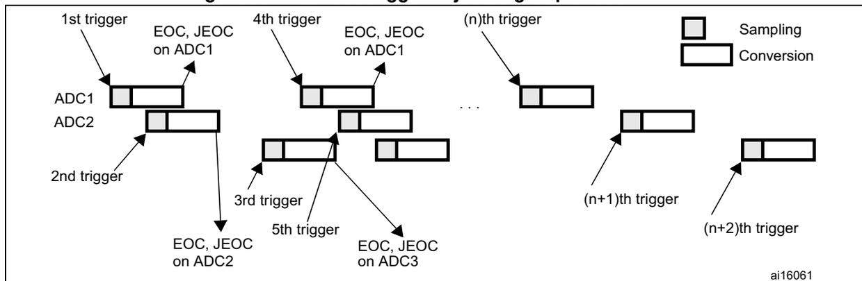
**13.9.5 Combined regular/injected simultaneous mode**
