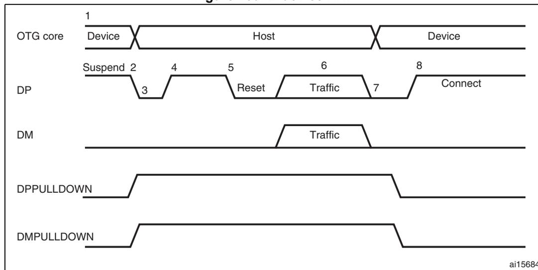
1. DPPULLDOWN = signal from core to PHY to enable/disable the pull-down on the DP line inside the PHY.
