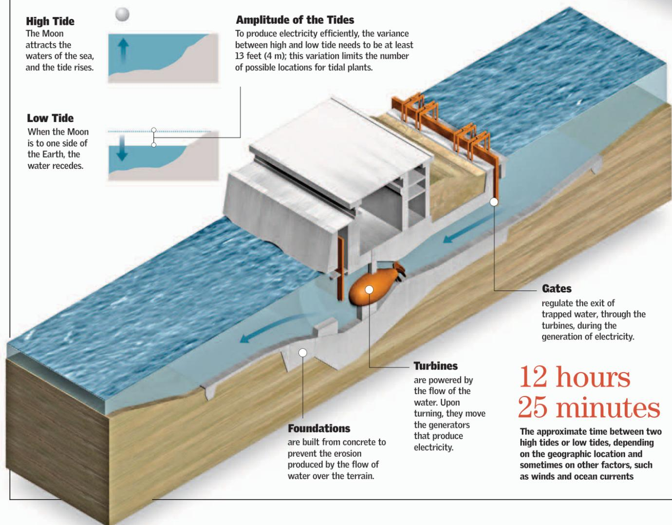
**Gates** are opened to let the water in as the tide rises and then closed to prevent its exit.
