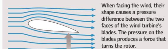
**Blades** measure, on average, 130 feet (40 m) in length. Three-blade rotors have proven to be the most efficient design.
