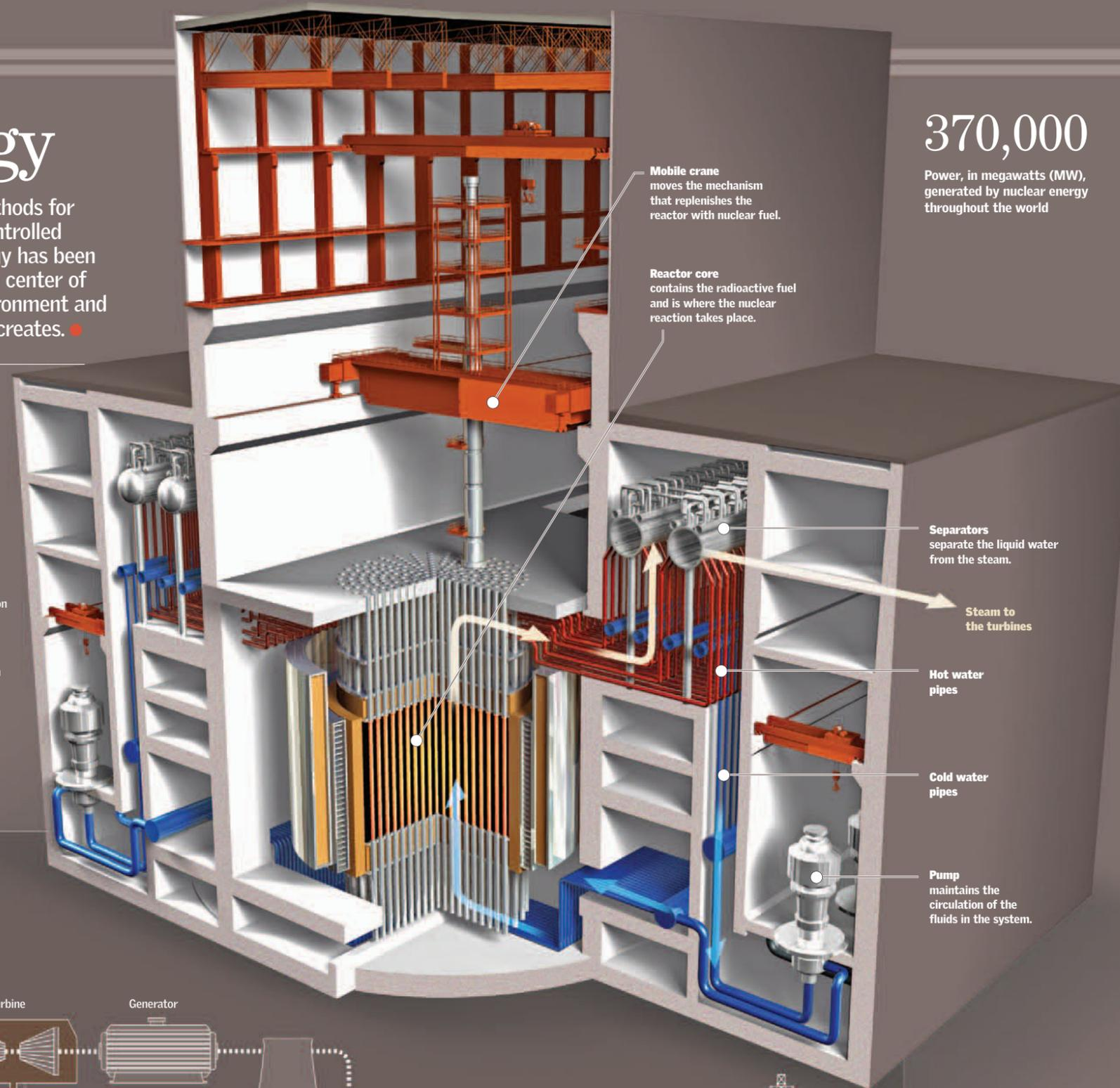
Mobile crane moves the mechanism that replenishes the reactor with nuclear fuel.
