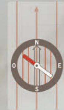
1 The compass is pointed toward the destination by aligning it with the baseline.
