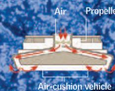
**HOVERCRAFT.** Since 1960. It uses propellers that produce an air cushion below the boat. Some ferries use this flotation system.
