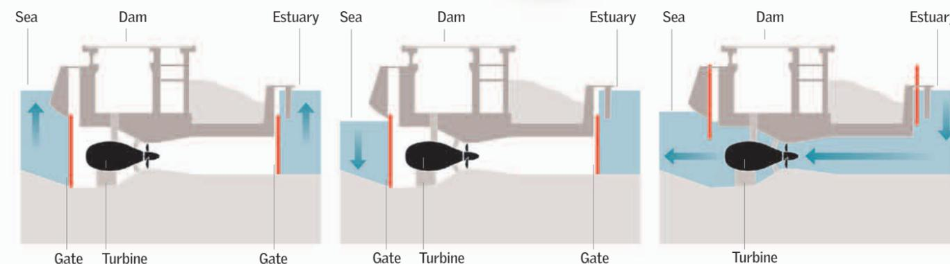
**1 High Tide** During high tide, the level of the water rises in the estuary. The gates of the dam are opened to let the water in.
