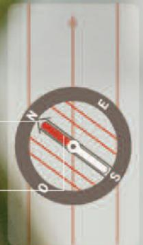
3 Keeping the pointer lined up with the needle ensures that the direction is maintained.
