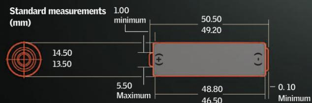
**POSITIVE TERMINAL** has the shape of a circular button.
