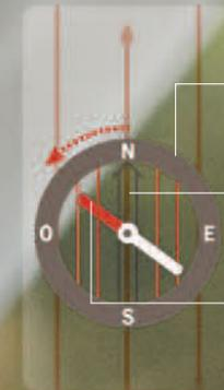
2 The graduated dial is rotated until the pointer is lined up with the magnetic needle.
