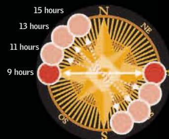
Foucault deduced that if the plane of oscillation of the pendulum cannot change, it was the Earth that revolved underneath the pendulum.
