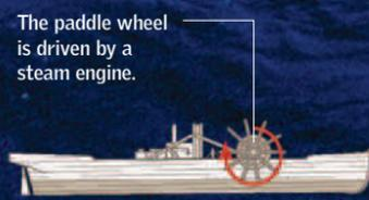
**STERNWHEELERS.** Beginning of the 19th century. Oldest ship propelled by an engine. The blades of the paddle wheel, acting like oars, cause the boat to move.
