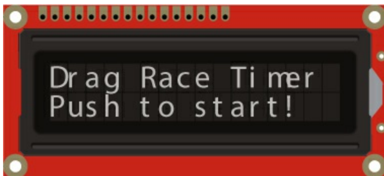
FIGURE 9-13: LCD display text at the start of the race
