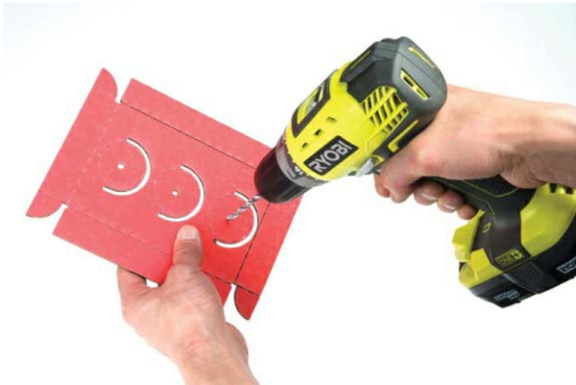
FIGURE 2-17: Drilling holes for the LEDs
