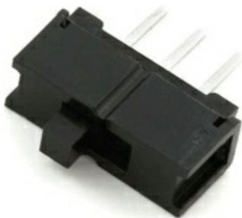
FIGURE 6-40: The single-pole, double-throw switch
