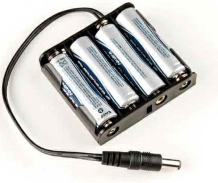
FIGURE 2-12: A 4 AA battery pack with a barrel jack adapter
