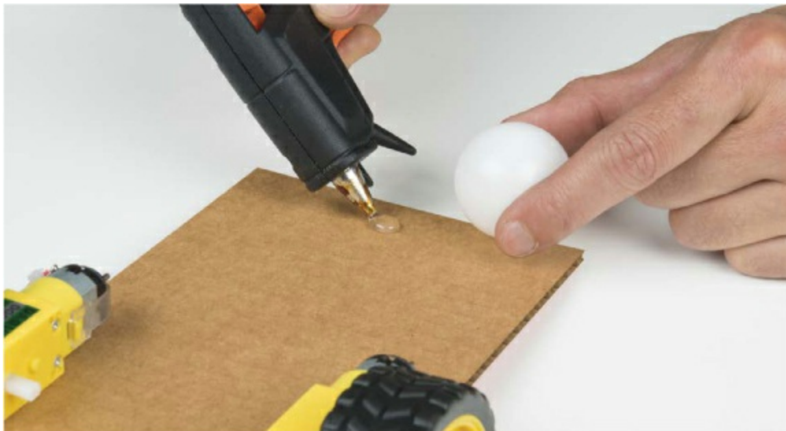
FIGURE 8-16: Attaching a ping-pong ball as a skid caster
