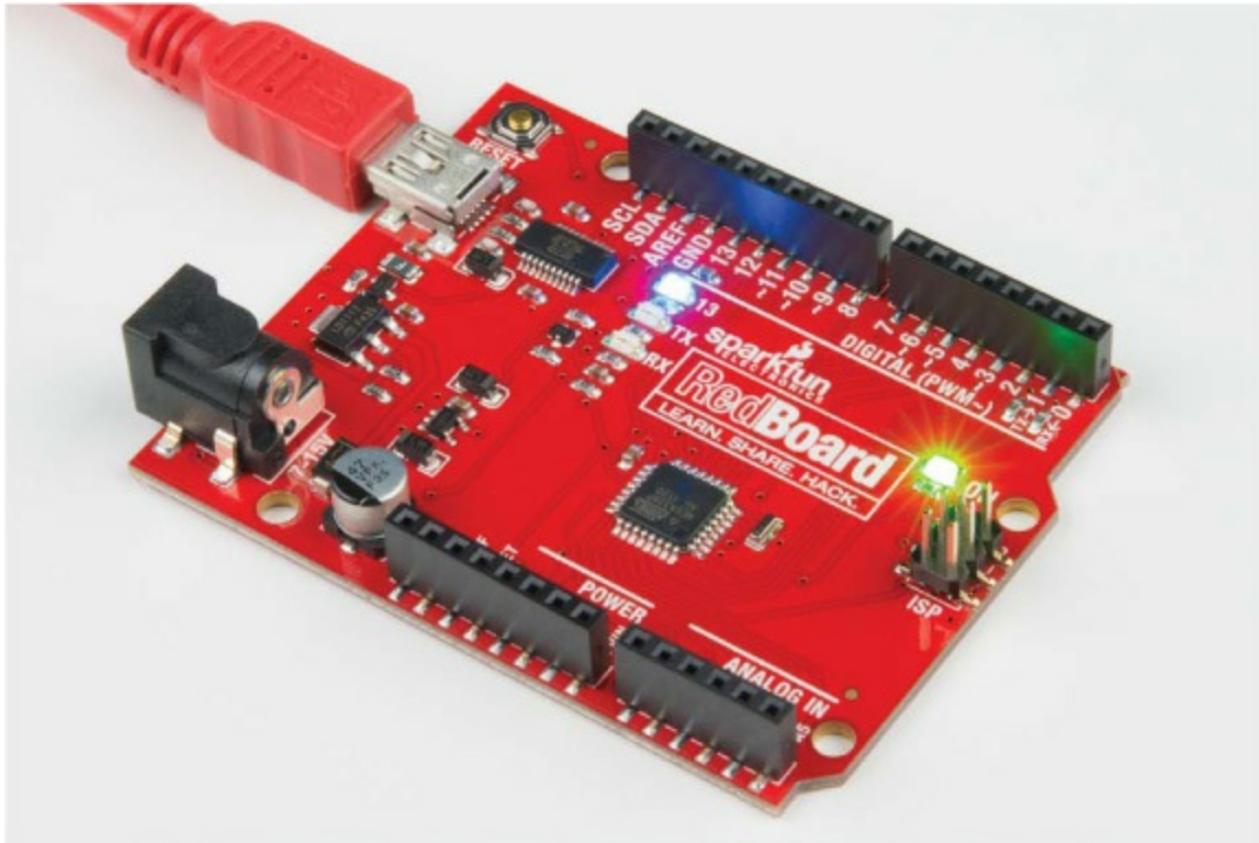
FIGURE 1-19: Turning on LED 13
