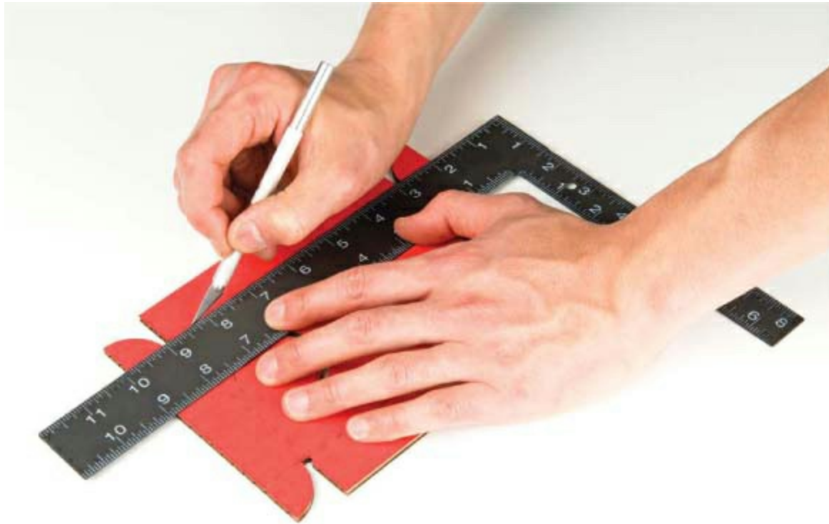
FIGURE 2-16: Scoring along the template with a craft knife and metal ruler
