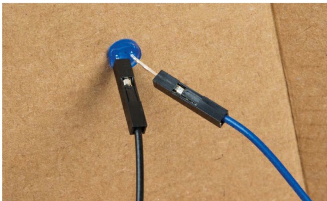
FIGURE 4-21: Connecting the LED to the jumper wires
