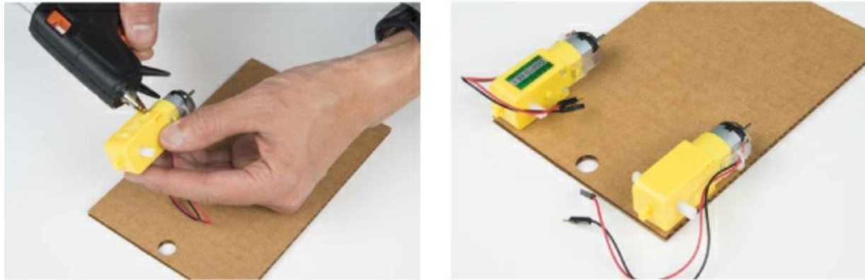
FIGURE 8-13: Attaching the motors to the chassis with hot glue
