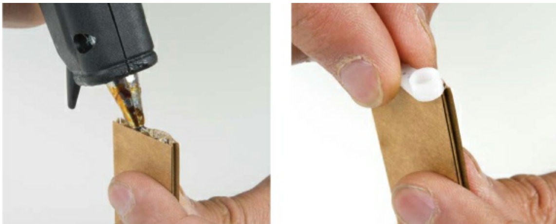
FIGURE 9-19: Gluing the servo horn onto the edge of the starting gate
