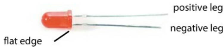
FIGURE 1-20: An LED showing the long and short legs
