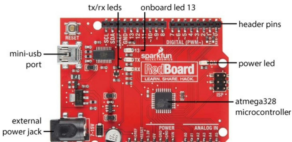
FIGURE 1-3: The Arduino-compatible SparkFun RedBoard. Notice how its shape matches up with the Arduino Uno in Figure 1-2 .
